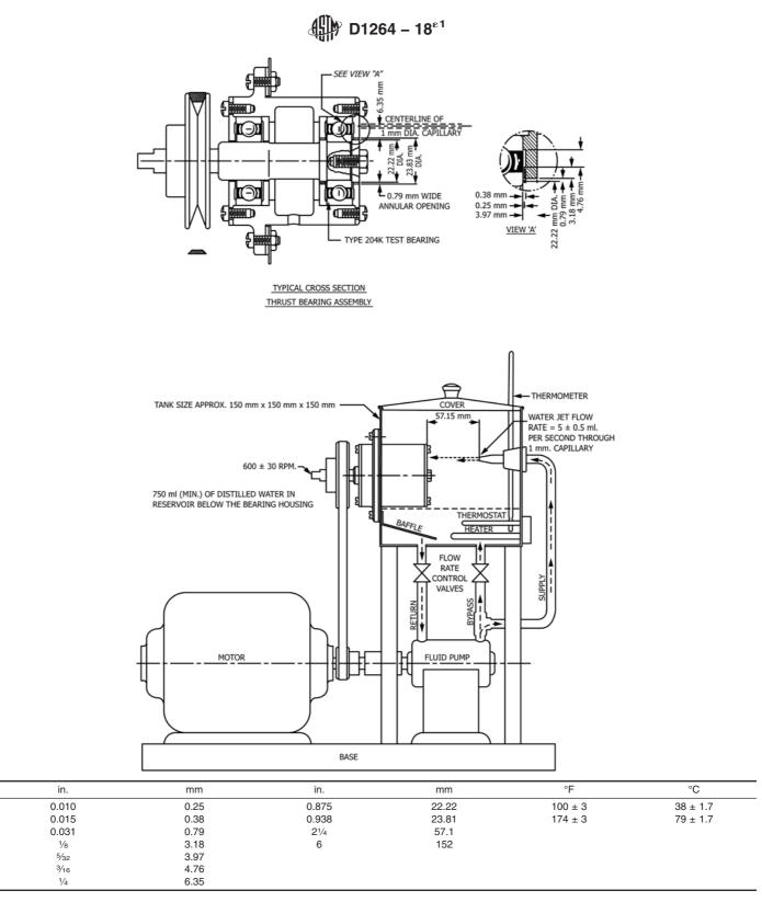
FIG. 1 Water Washout Characteristics of Lubricating Grease Apparatus
